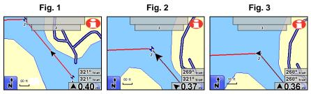
Navigating a route made from a trail. Fig. 1 shows boat on first leg of the route. In Fig. 2 boat nears point two and unit automatically switches navigation to point three. Boat is still tracking 321°, but bearing overlay now shows point three is 269° away. Steer arrow also swings left, showing which way to turn. Fig. 3 shows boat has turned on new course. Boat track is 268° which now matches the bearing to point three which is 0.36 mile away. Steer arrow points straight ahead.
